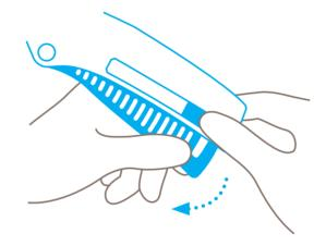
Swing the lever completely **out of the handle** and flip open the blade cover.
