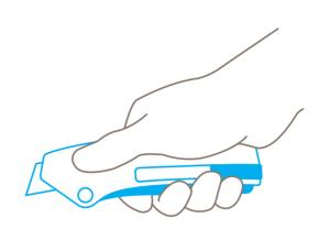
To **engage the blade**, unlock the cutter and squeeze the lever. Now you can cut.
