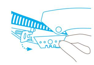
Now you can either **rotate or replace** the blade. Re-close the blade cover.
