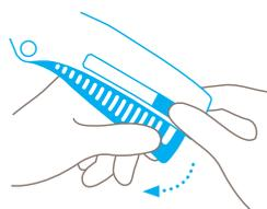
Swing the lever completely **out of the handle** and flip open the blade cover.
